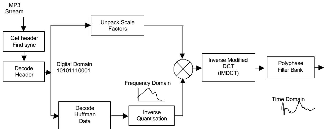
Figure 1. MP3 Processing Stages
