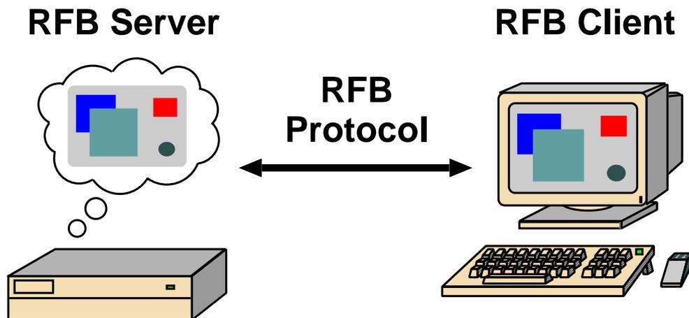
RFB is truly a “thin client” protocol. The emphasis in the design of the RFB protocol is to make very few requirements of the client. In this way, clients can run on the widest range of hardware, and the task of implementing a client is made as simple as possible.
