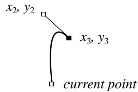
$x_2\ y_2\ x_3\ y_3\ \mathbf{V}$  The **V** operator is similar to the **v** operator, but the new current point is a corner.
