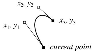
$x_1\ y_1\ x_2\ y_2\ x_3\ y_3\ \mathbf{C}$  The **C** operator is similar to the **c** operator, but the new current point is a corner.
