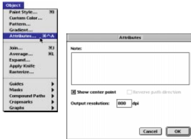
*showCenter* **Ap** – The **Ap** operator determines whether or not the center point of a path is displayed. By default, only rectangular (including square) and oval (including circular) paths have visible center points, but the center point of any path can be displayed by setting the value of the *showCenter* argument
