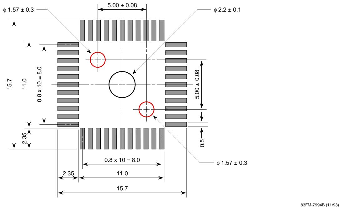
**EV-9200G-64 Socket Dimensions**
