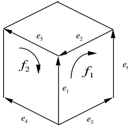
Figure 5.2.1.3 – Edge and face orientations for a cube.
