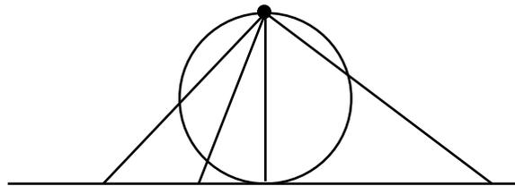
Figure 5.2.3.8 – Projecting a sphere on a plane using the North pole as the viewpoint.
